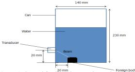
**Figure 1.** Canned food specimen and experimental setup
